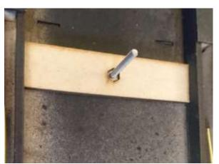
Insert the bolt head into the hexagonal cut out
