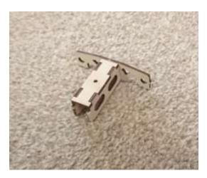
Attach the stretcher bar side plates into one of the side frames for each bogie, (you may need to sand the end a little to fit).
