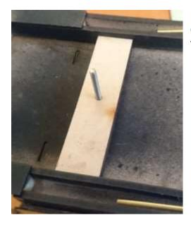
Glue the second strip with the 3mm hole over the first strip to captivate and retain the bolt.
